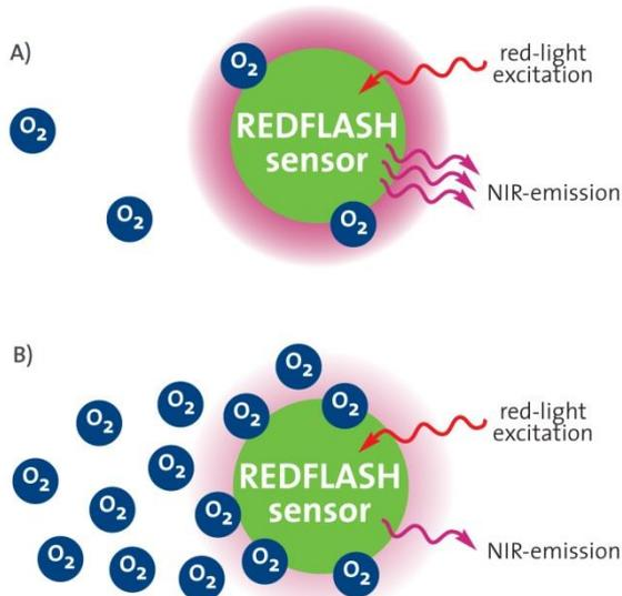
Principle: red light excited REDFLASH indicators show luminescence in the near infrared (NIR), which decreases with increasing oxygen (quenching effect).
