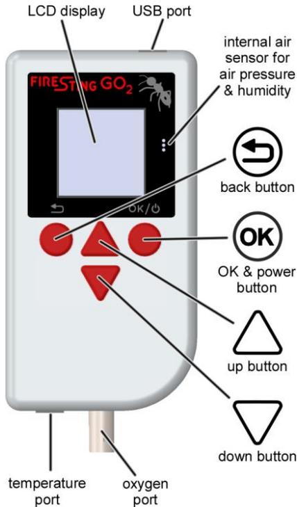
The user interface of the **FireSting-GO<sub>2</sub>** consists of the display and four buttons:
