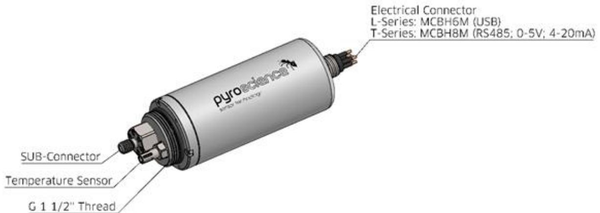
The housing is dependent on the chosen device. **APHOX-TX** comes with a titanium housing for deployments down to 4000m. **APHOX-T-PH** and **APHOX-T-O2** come with a POM housing capable for deployments down to 100m.
