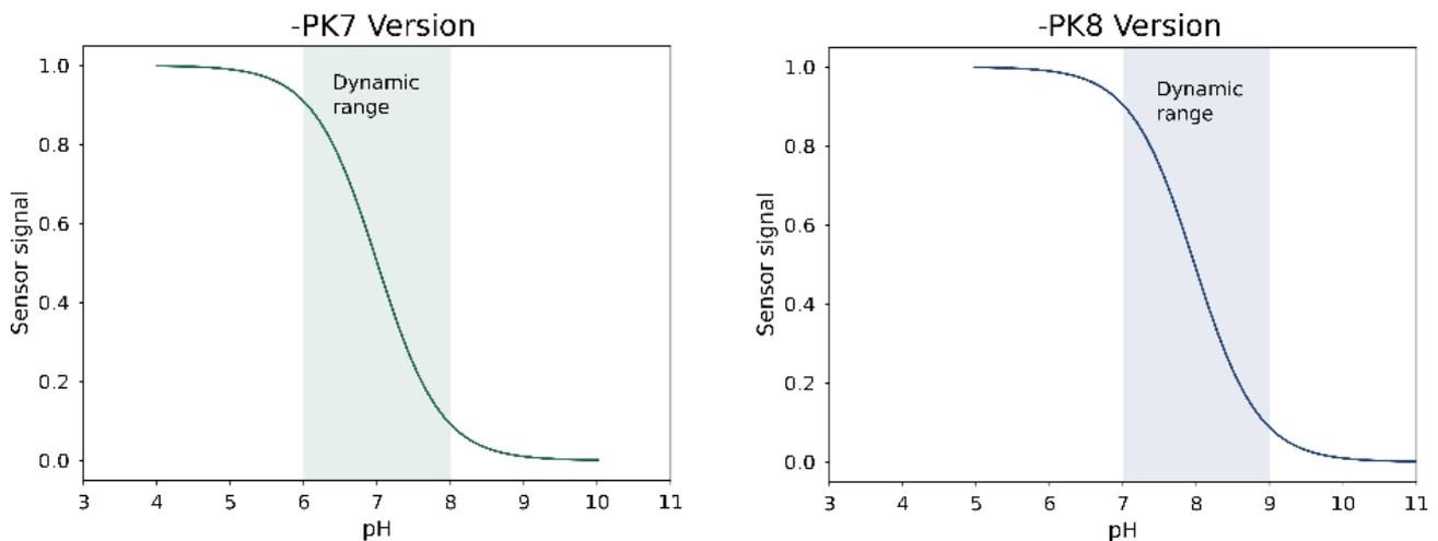
Calibration of both versions is performed at low pH values (completely protonated indicator dye) and at high pH values (completely de-protonated indicator dye). For this reason, it is possible to use the same pH buffer capsules (**PHCAL2** and **PHCAL11**) for both pH sensor versions.
