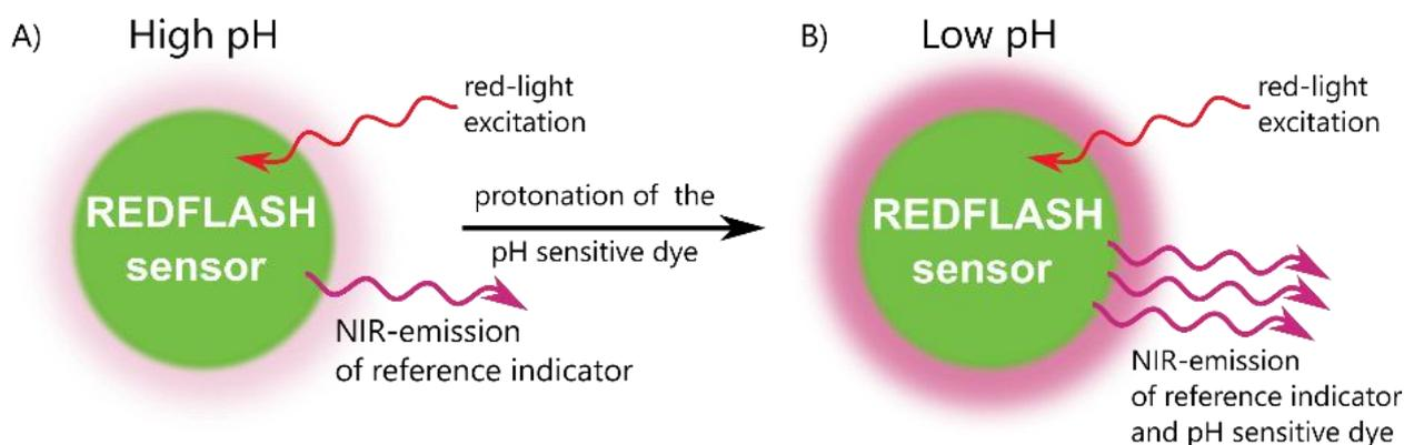
**Principle:** red light excited REDFLASH sensor shows luminescence in the near infrared (NIR). The REDFLASH sensor consists of a pH insensitive reference indicator and a pH sensitive dye. **A)** low NIR emission from just the reference indicator and **B)** high NIR emission from the protonated dye and the reference indicator.
