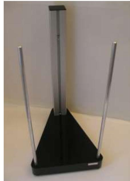
5. There are four mounting nuts integrated in the grooves on either side of the main post. They provide a M6 thread for mounting micromanipulators. The mounting nuts are spring loaded; their vertical position can be adjusted by sliding them up and down.
