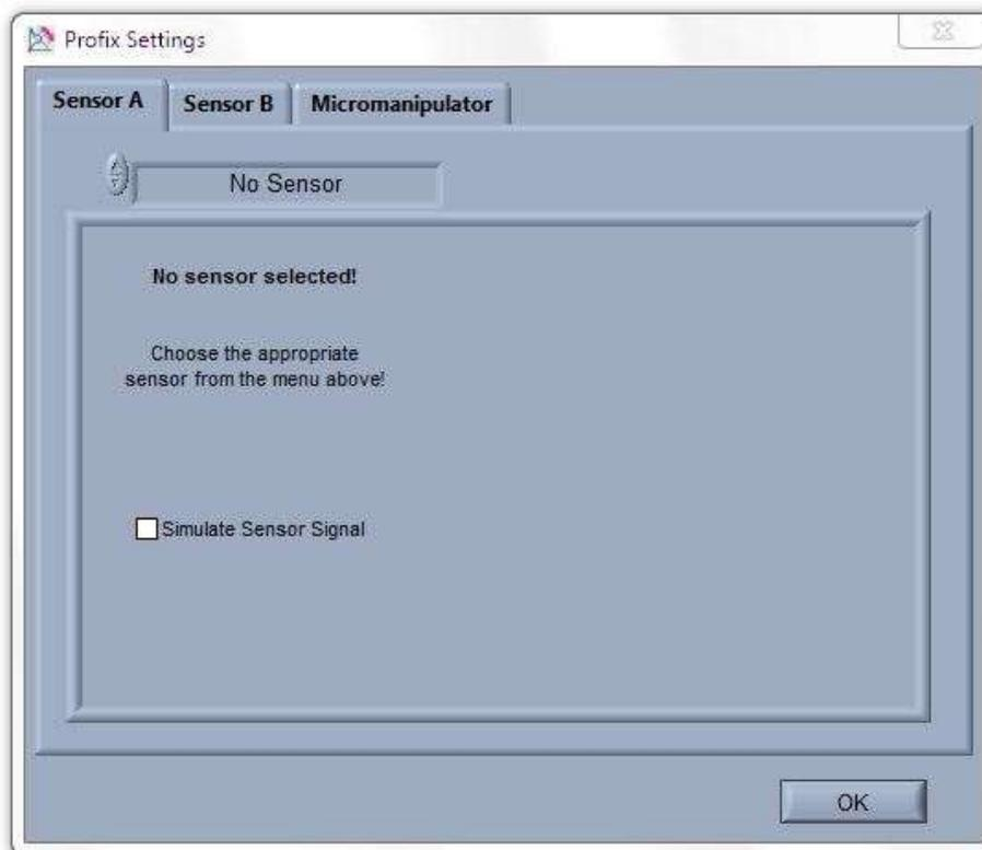
**Profix** reads up to two microsensor signals, which are designated within the program as **Sensor A** and **Sensor B**. In the tabs **Sensor A** and **Sensor B** of the **Profix Settings**, different fiber-optic meters (e.g. **FireSting**) can be selected. If only one microsensor will be used, just leave one channel (e.g. Sensor B) as "No Sensor".
