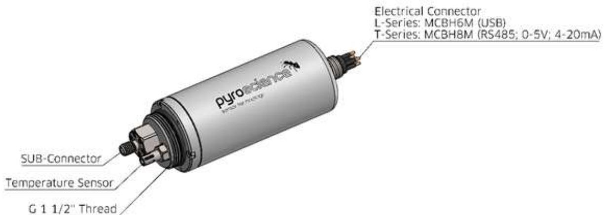
The housing is dependent on the chosen device. **APHOX-LX** comes with a titanium housing for deployments down to 4000m. **APHOX-L-PH** and **APHOX-L-O2** come with a POM housing capable for deployments down to 100m.
