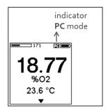
In the PC Mode, only the UP and DOWN buttons are active for scrolling between top and sub-screens of the Live Mode. Access to the menu is blocked. However, now the **FireSting®-GO2** meter can be controlled completely by the **FireSting®-GO2** Manager software on the PC. It offers an extended functionality compared to the LCD user interface, including log file download, log file deletion, and log file inspection.
