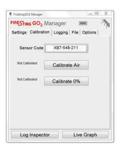
For highest precision it is recommended to calibrate both calibration points. However, if the expected measuring range is close to one of the calibration points, then a 1-point calibration might be sufficient. For example, if the expected measuring range in a liquid sample is 95-100% air sat., then a 1-point calibration at air saturated water is typically sufficient. In this case the 0% calibration is taken from the factory calibration encoded in the **Sensor Code**.
