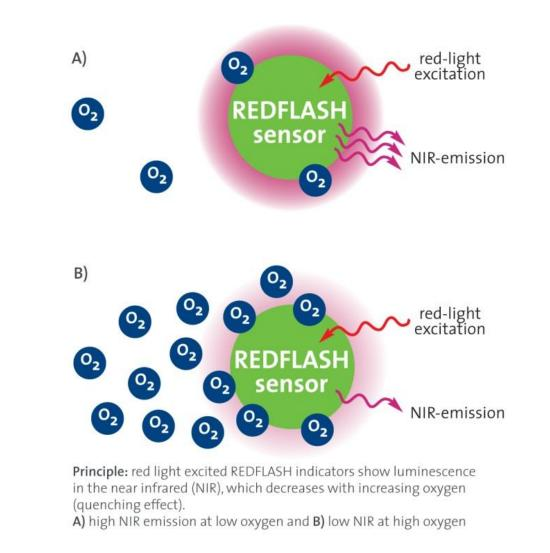
The **REDFLASH technology** impresses by its fast response times, high precision, high reliability, low power consumption and low cross-sensitivity. The red light excitation significantly reduces interferences caused by autofluorescence and reduces stress in biological systems.
