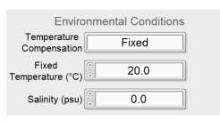
performed with a fixed sample temperature. In this case the temperature needs to be measured in the sample and entered as **Fixed Temperature** (°C).
