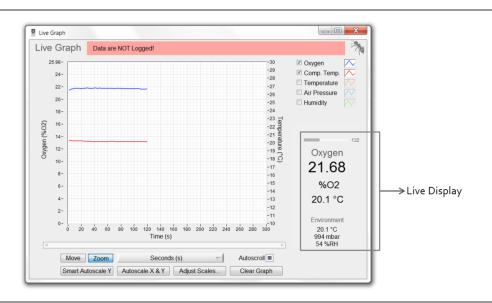
The Live Display shows numerical live readings of all sensors comprising oxygen, compensation temperature, temperature (if a temperature sensor is connected), and the readings of the internal air sensor (air pressure, relative humidity).
