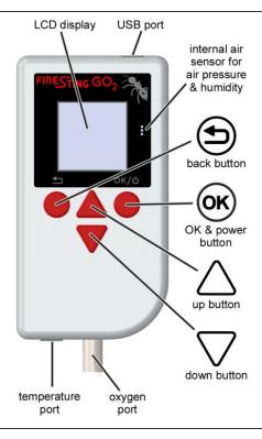
The user interface of the **FireSting-GO2** consists of the display and four buttons:
