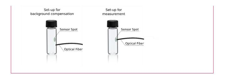
Please ensure that **during the subsequent calibration process** the **Optical Fiber** is again **attached to the medium WITH** oxygen nanoprobes or to the position with sensor spots.
