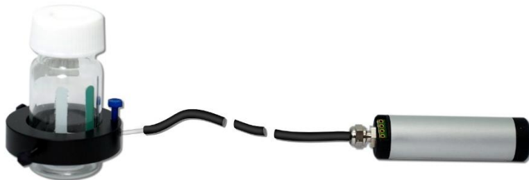
Figure 4: Connection of a pH vial to Pico-pH via an optical fiber.
