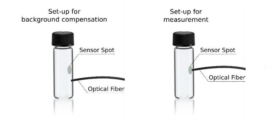
Please ensure that **during the subsequent calibration process** the **Optical Fiber** is again **attached to the medium WITH** oxygen nanoprobes or to the position with sensor spots.
