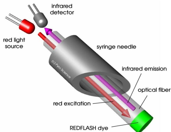
The measuring principle is based on a sinusoidally modulated red excitation light. This results in a phase-shifted sinusoidally modulated emission in the NIR. The **PyroScience** read-out device measures this phase shift (termed "**dphi**" in the software). The phase shift is then converted into oxygen units based on the Stern-Vollmer-Theory.
