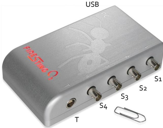
Depending on the purchased version, the *FirestingO<sub>2</sub>* is equipped with 1, 2, or 4 channels (receptacles S1 to S4) for fiber-optic oxygen sensors and one receptacle (T) for a PT100 temperature sensor. The USB-connector provides the energy supply and the data exchange with the PC. The device is operated by the Windows software *Oxygen Logger* provided by *PyroScience*.
